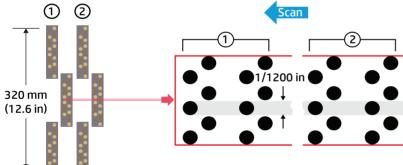
HP Metal Jet printers use six printheads arranged in two **printbars** on the print carriage
