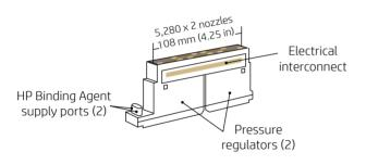
Each printhead produces a 108-mm (4.25-inch) print swath with two independent columns of 5,280 nozzles that are spaced 1200/inch in each column. There are **two** independent supply ports for HP Binding Agent and two built-in pressure regulators.
